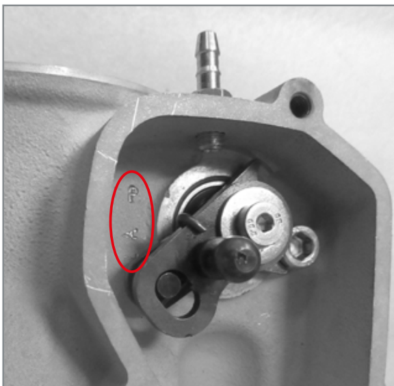
Cylinder class punching.
