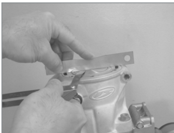
Case where the plate and piston do not touch: check distance between plate and piston.
