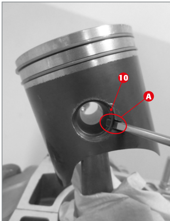
Removal of piston circlip.
