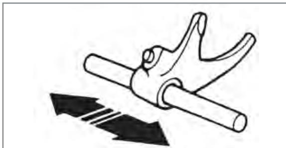
Check fork sliding on pin.
