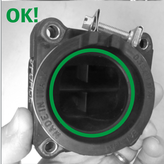
Flow guide positioning.
