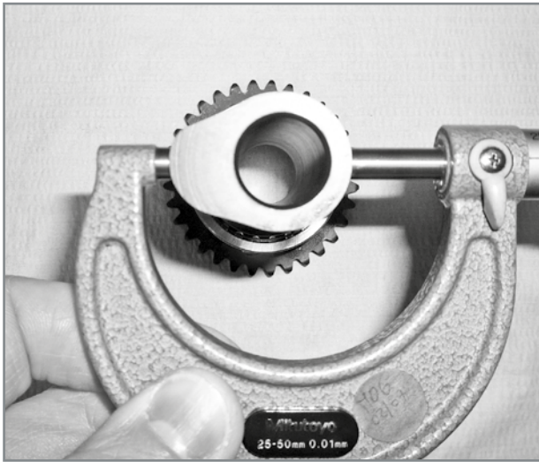
Cam height measurement.
