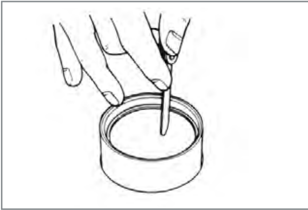
Elastic band wear limit check.
