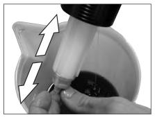
Move the pumping unit and drain the remaining oil. When the oil has been drained completely, introduce the amount of new oil described in chapter 1.
