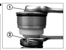
• Loosen the counter-nut 2 and remove cap 1.
