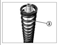
• Extract the spring **3** and overturn the pipe, making the oil escape.
