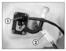
Disconnect the electrical connector **1** and **2**
