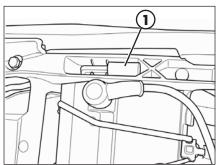
The hex key **1** and its socket wrench (8 mm) are found inside the battery compartment. Remove the seat to reach them (page 80).
