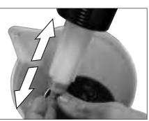
• Move the pumping unit and drain the remaining oil.
