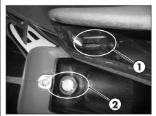
To re-assemble: Insert the cavity **1** of the saddle in slot **2**.
