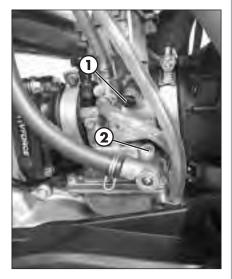
• Tighten the air adjustment screw no. 2 fully and then loosen it up to the value described in the carburetor setting table (page 13)
