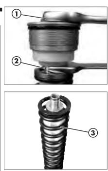
• Loosen the counter-nut **2** and remove cap **1**.
