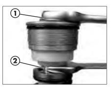
• Bleed the pumping unit of air, making it rise and fall until complete loading. Introduce the spring and screw the cap **1** until it is completely inserted on the pumping rod. Block the cap to the pumping rod via the counter-nut **2**.
