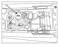
To open the fuel tank cap turn it anticlockwise.
