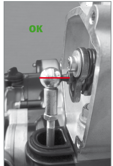
Correct position of the control rod seat.
