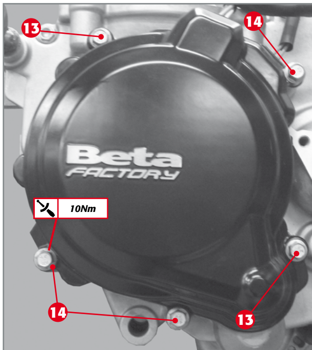
Flywheel cover coupled to crankcase.
