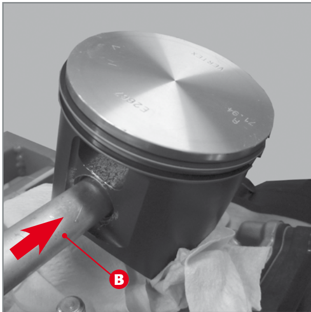
Removal of pin bolt.
