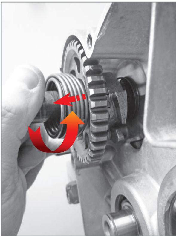
Extraction of shaft from crankcase.
