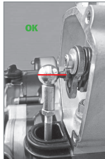
Correct position of the control rod seat.
