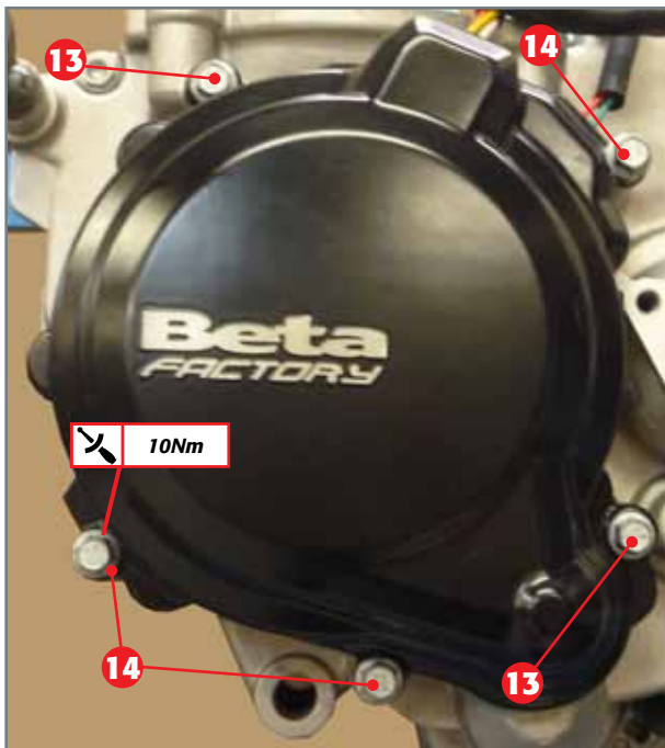
Flywheel cover coupled to crankcase.
