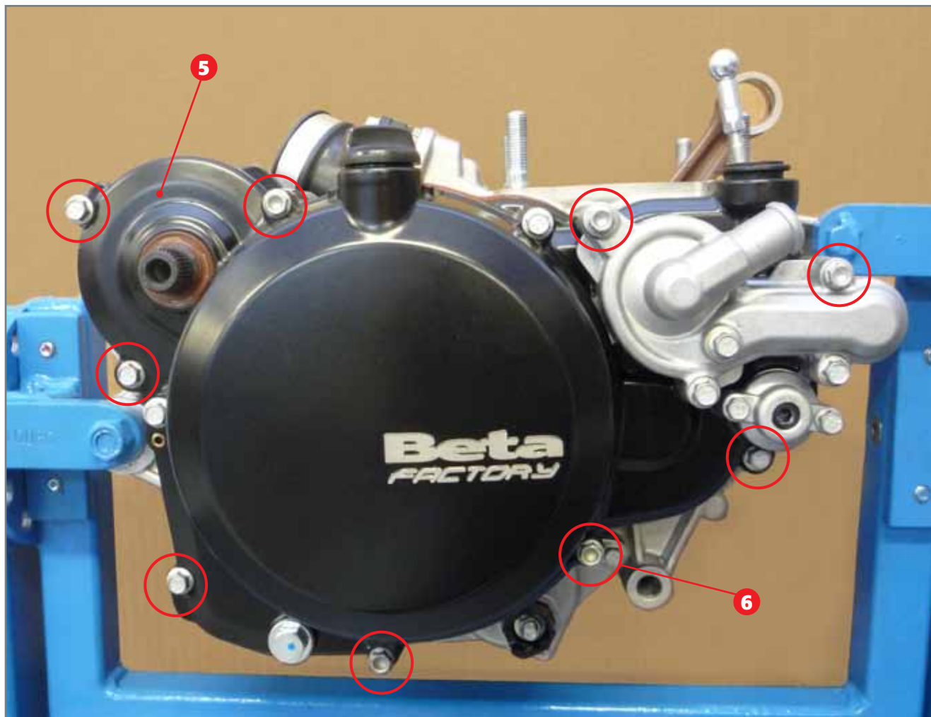
Inner clutch cover screws.
