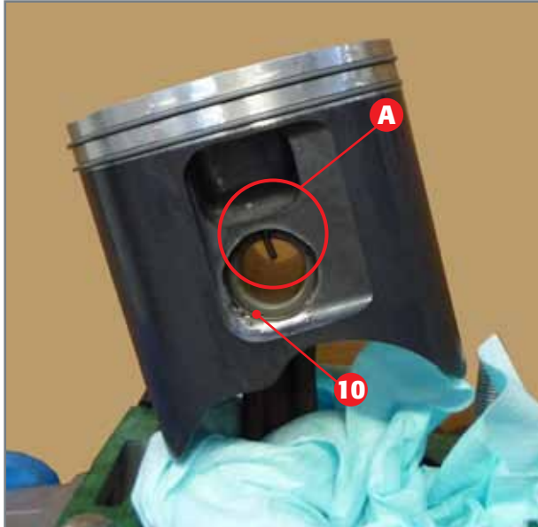
Removal of piston circlip.
