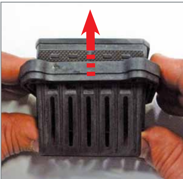
Disassembly of reed valve body.
