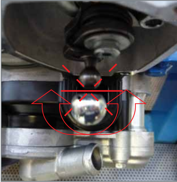
Check of control rod rotation.
