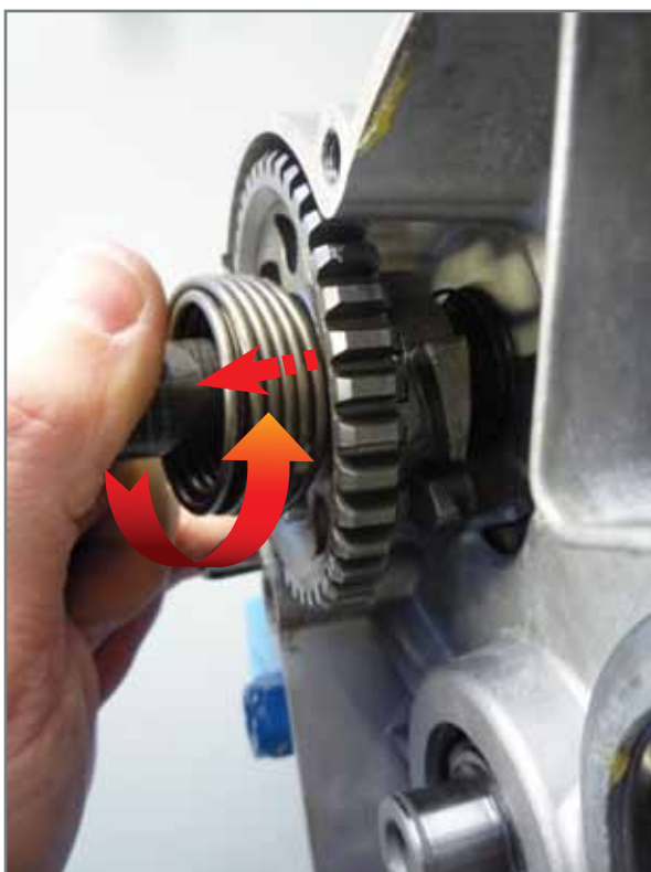
Extraction of shaft from crankcase.
