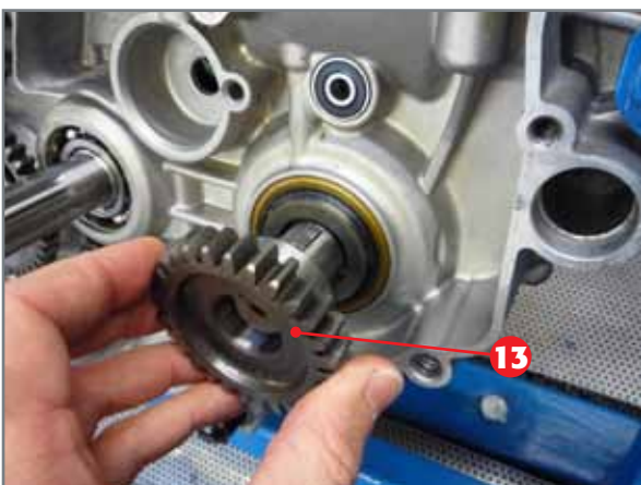
Removal of main gear.
