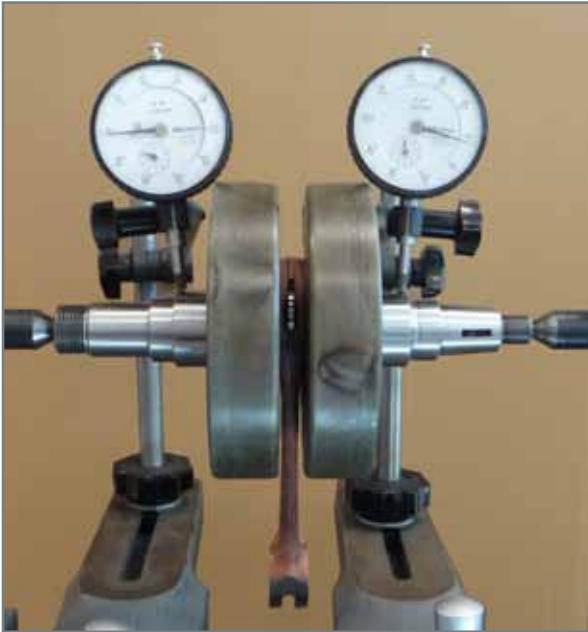
Deflection/Off-centring of crankshaft.
