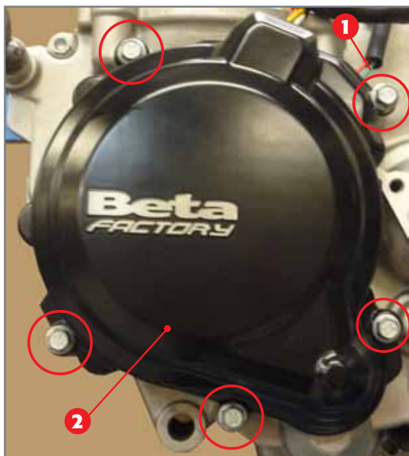
Fixing screws 1 of flywheel cover 2.
