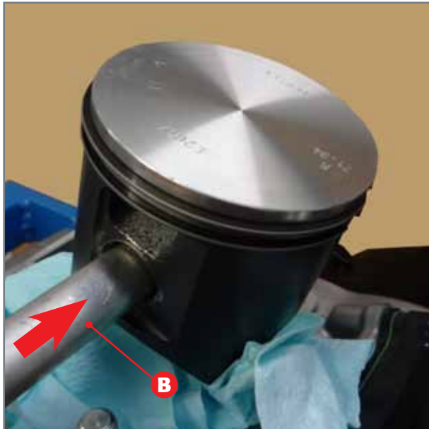
Removal of pin bolt.
