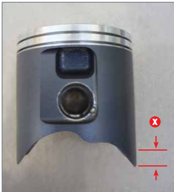
Quota at which to measure the outside diameter of the piston.
