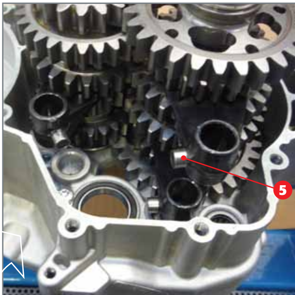
Extraction of forks from gearbox unit.
