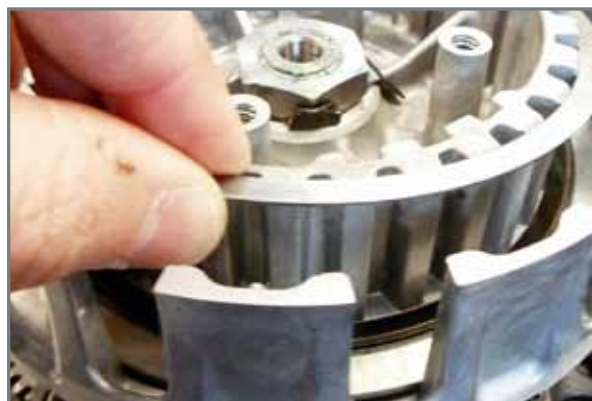
Removal of disc spring assembly.
