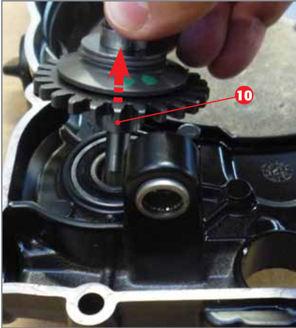
Extraction of centrifugal unit.
