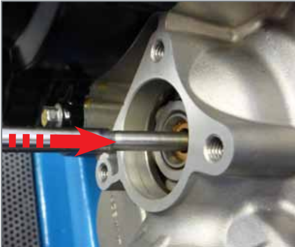
Insertion of clutch rod.
