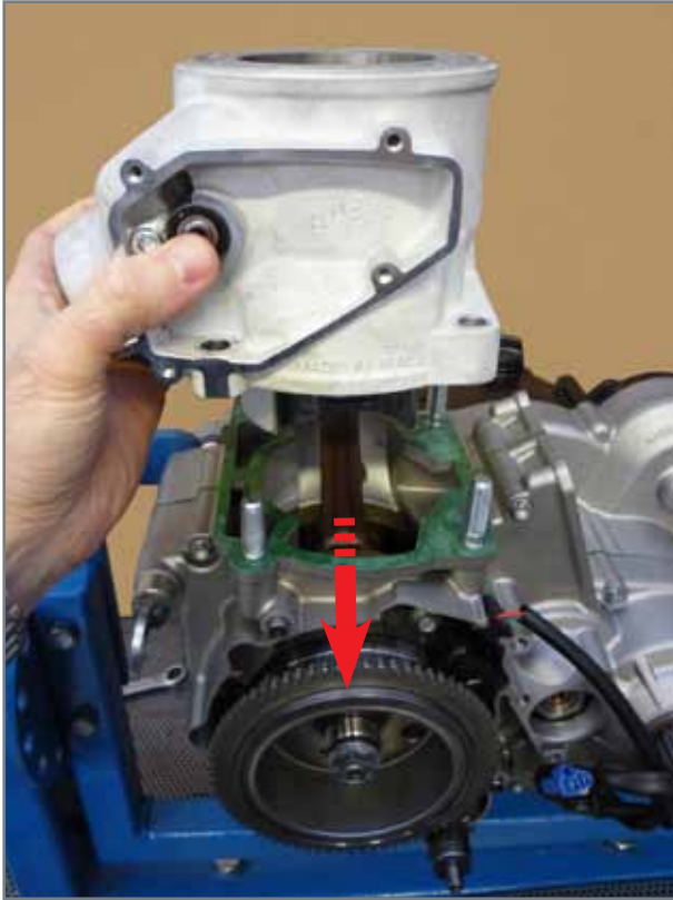
Coupling of cylinder to piston and crankcase-
