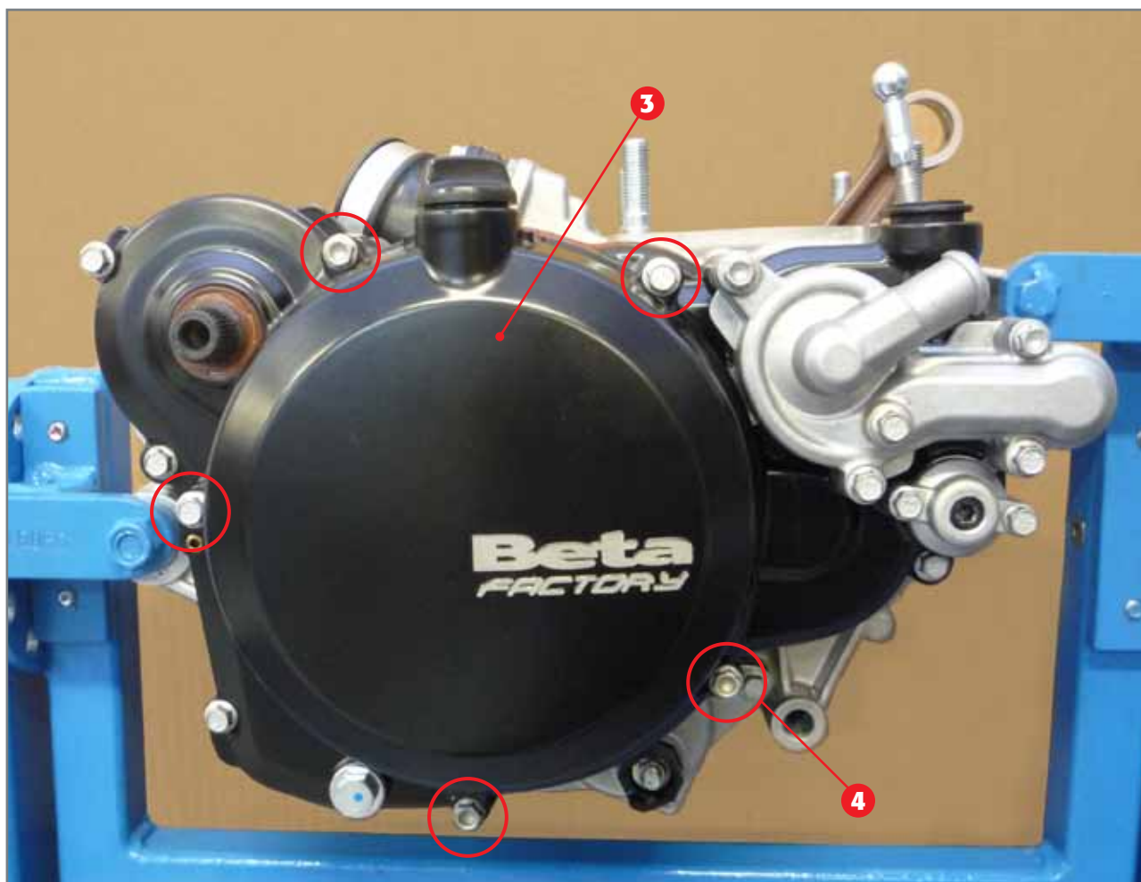
Outer clutch cover screws.
