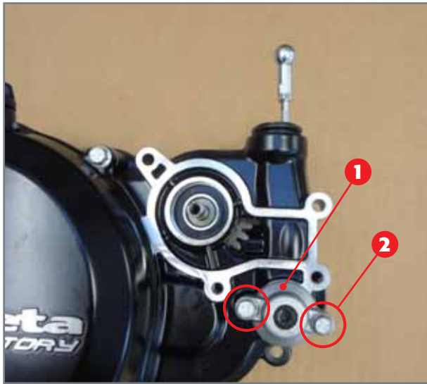
Removal of centrifugal adjustment cover.
