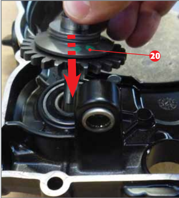
Insertion of centrifugal.
