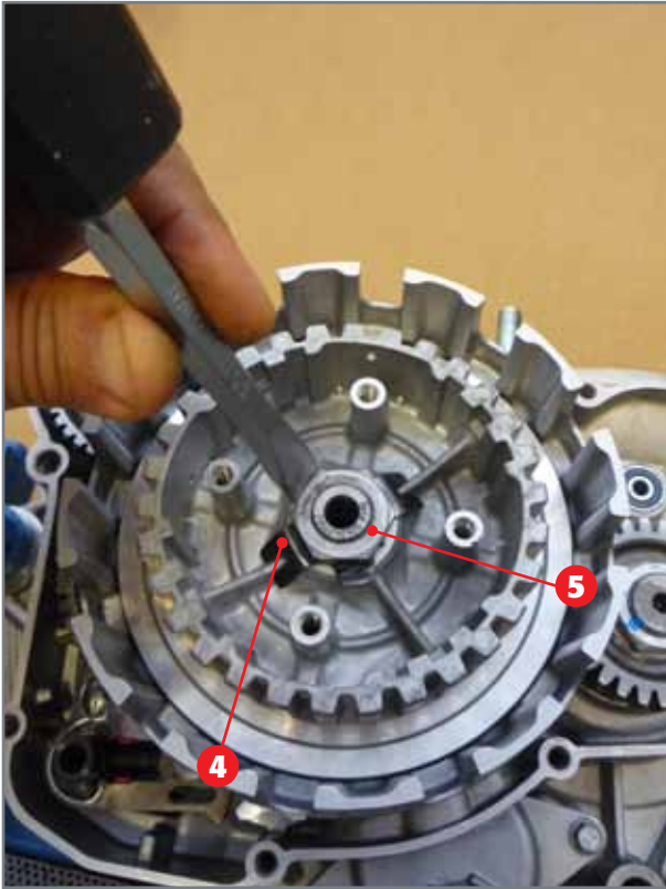
Opening of the safety washer with chisel.
