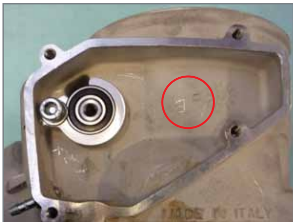
Punching of cylinder class.
