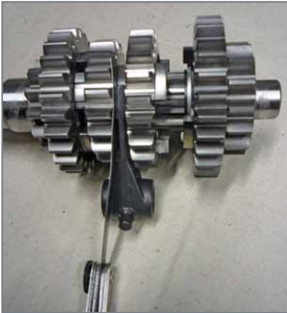
Check of wear of forks and gearwheels.
