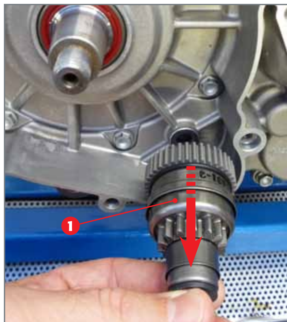
Removal of Bendix coupling.
